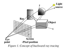
Backward ray tracing is where rays are cast from the eye into the environment. As such, backward ray tracing, as shown in Fig. 1, identifies incident light energy based on tracing rays from the eye as the point of observation to the screen as the viewing space.<sup>4.5</sup> Therefore, the algorithm is very efficient and can reduce the computational cost, as it only traces the number of rays as fixed by the resolution size.
