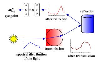
Figure 2. Calculation of color based on spectral distribution of light sources and objects
